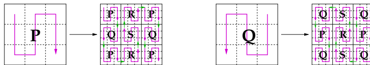
Fig. 1. Recursive construction of a Peano curve (for patterns P and Q , only)
